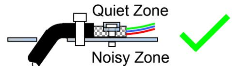
3. "Pigtail" the screen to a suitable earth point. Ensure the pigtail length is as short as possible.
