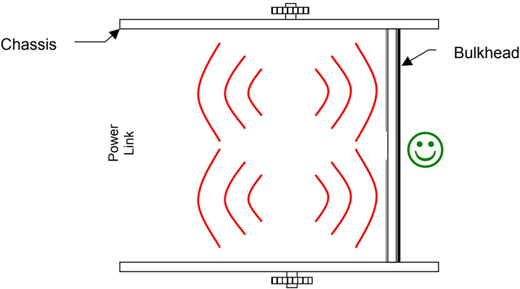
If you can't avoid running the sensitive cables past the nasty stuff, then they will probably need screening; this is effectively an extension of the Faraday cage. The screen will need to cover as much of the cable as possible.
