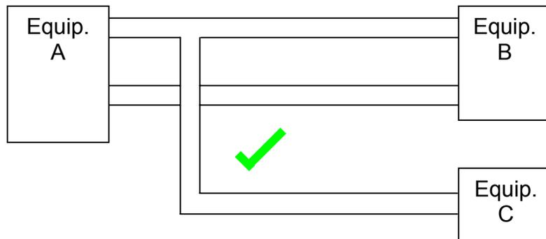
However, whilst maintaining separation, try to ensure that wiring between the same pieces of equipment follows a common route; else you could be in danger of creating a loop that could pick up noise.
