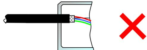
5. Pigtail termination too long. Ideally the pigtail should be no longer than 5 times its width.
