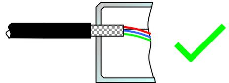
2. Saddle-clamp the screen to a bulkhead immediately inside the "Quiet Zone".
