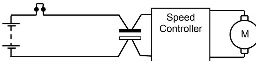
The capacitor is essentially a small reservoir, its purpose is to supply current when needed, absorb small surges from re-gen braking and soak up high frequency noise.
