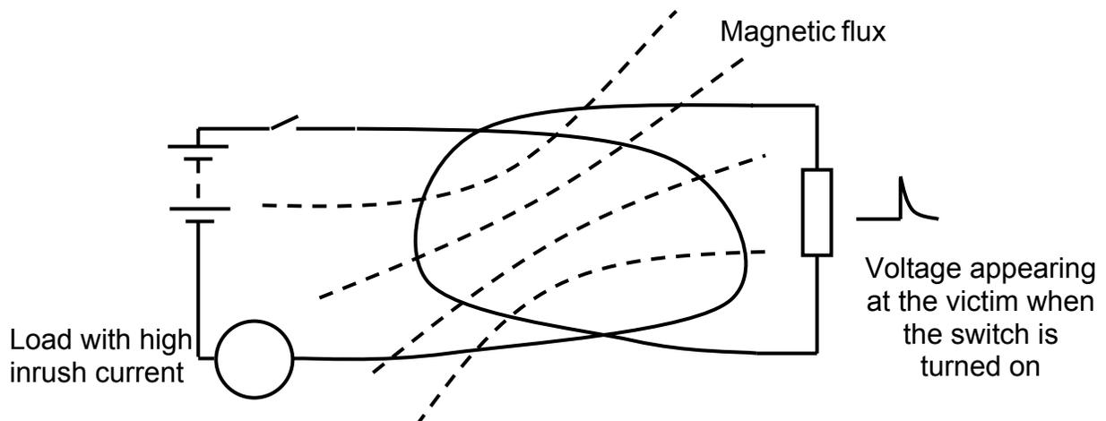
The amount of energy involved with this type of interference in particularly bad installations can destroy sensitive electronics.
