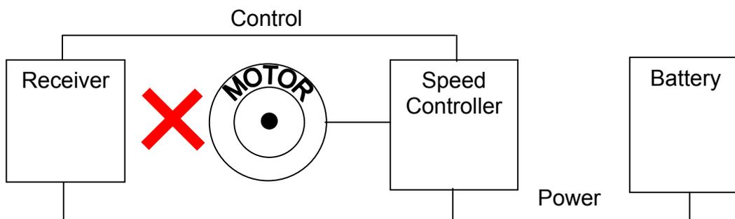
A word of caution, Do not be tempted to loom cables together just because they “Look Neat”, provided that the send and return cables run together a “Rats’ Nest” arrangement can work well, it’s just harder to maintain.
