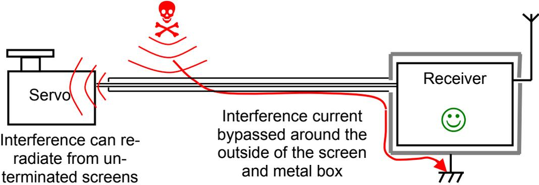
The above diagram shows a screen earthed at one end and free at the other; this runs the risk of letting the interference re-radiated onto the system and wiring at that end, then being conducted back along the signal wires to the receiver.
