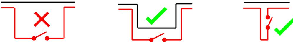
Better still, **twist the send and return wires together** and the net magnetic flux through adjacent turns will cancel each other (provided the twists are even); it will also even out the charge on the wires if subject to an electric field. The intention of this is to reduce the interference between the lines. **The tighter the twists the better.**
